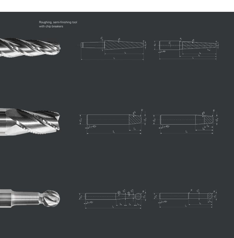
Starrag offers the biggest choice of tools specific for Impeller machining. For flank milling open Impeller airfoils in one go, taper ball nose cutters up to 50mm in diameter and 600mm in length are available with or without chip breakers. For every Impeller – from car
